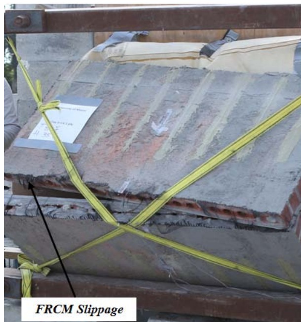
(e) (Fabric breaks because of collapse)
