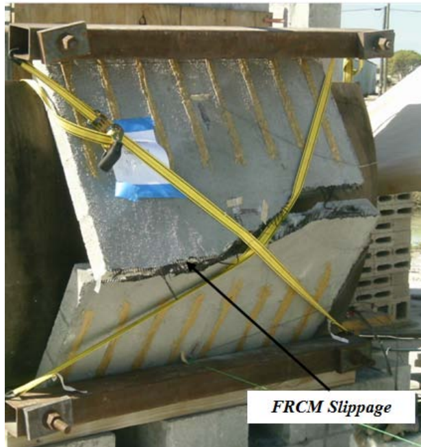
(b) (Fabric breaks because of collapse)
